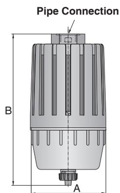
These are integral air-silencer and oil-separation devices. When installed at the exhaust ports of pneumatic valves, they capture over 90 per cent of the exhausted lubricants. They also reduce exhaust noise substantially. These units help to meet requirements for noise and oil mist control and have been approved globally by a number of reputed manufacturers.
