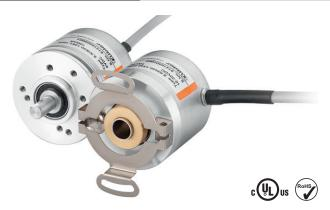
The incremental encoders type Sendix Base KIS40 / KIH40 with optical sensor technology have been designed for highest cost-effectiveness. They are available with a resolution of up to 2500 pulses per revolution.
