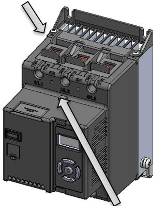
Step 2. Remove blanking plug (x1)
