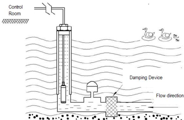
Fig. 08 – Damping device
