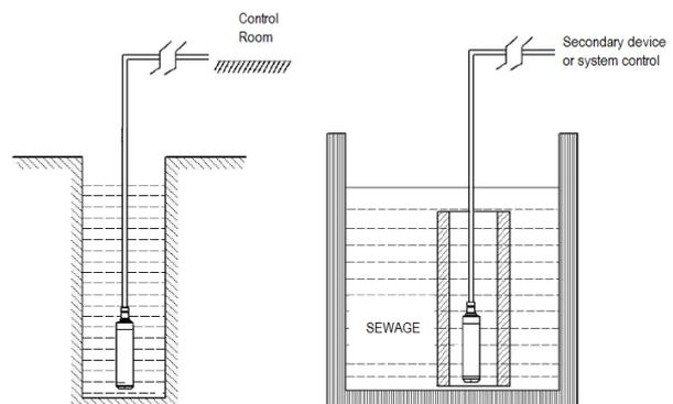
Fig. 06 – Still water installation
