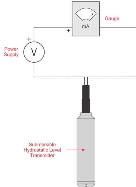
Fig. 05 – Electrical connections
