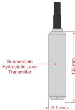
Fig. 03 – Transmitter dimensions
