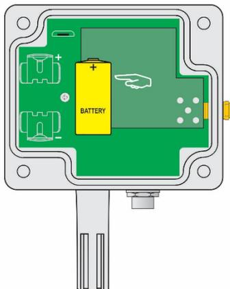
Figure 11 – Inserting the battery
