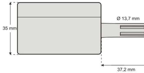
Figure 4 – RHT-Air measurements
