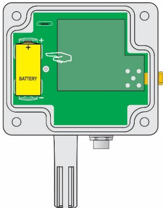
Figure 10 – Battery replacement
