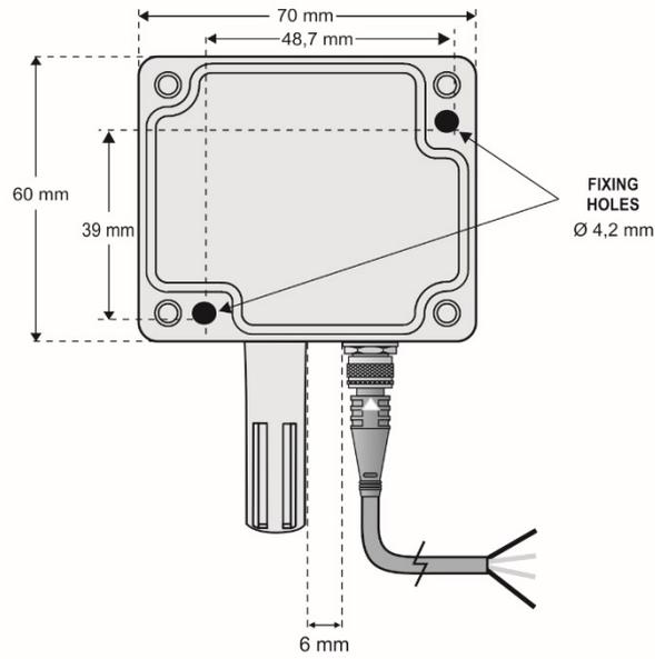
Figure 3 – RHT-Air mounting holes and measures
