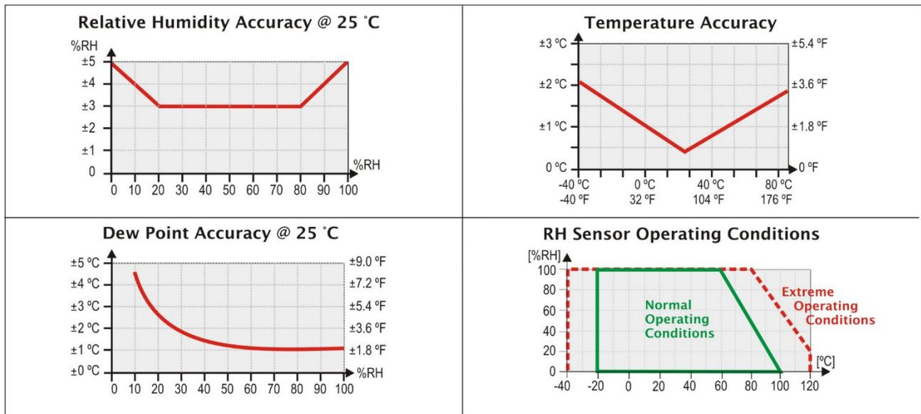
Figure 17 – Accuracy of the humidity and temperature measurement
