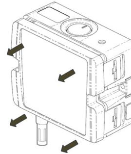
Figure 19 – Removing the front cover of the transmitter
