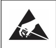
The sensor used in the RHT *Climate* Transmitter is a device that is sensitive to electrostatic discharge (ESD). Whenever the sensor is touched, measures need to be taken to prevent ESD damage.
