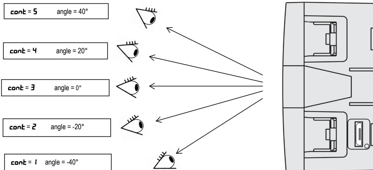
Figure 24 – RHT Climate Transmitter display contrast
