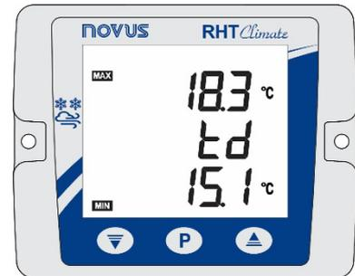
Figure 7 – Maximum and minimum dew point temperature
