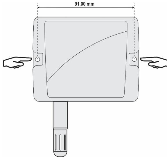
**Figure 14 – Mechanical Installation**
