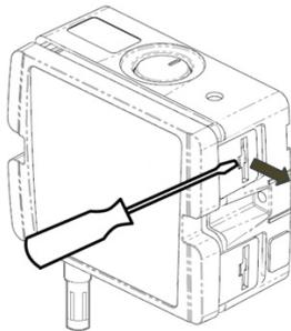
Figure 18 – Removing the front cover of the transmitter
