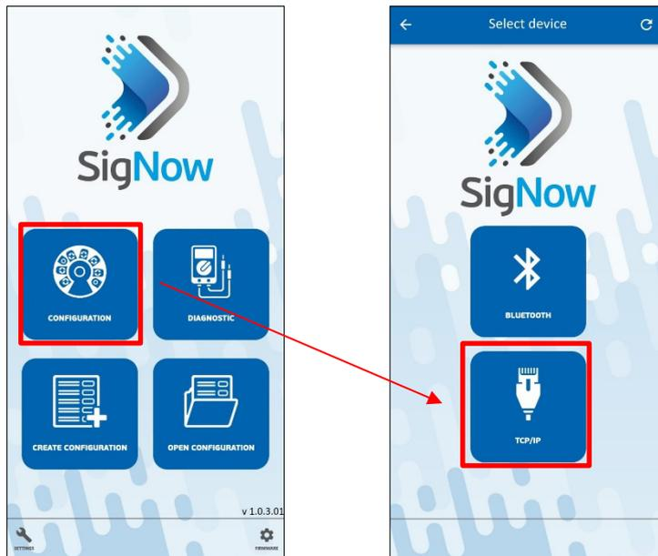
Figure 32 – Establishing a TCP/IP connection
