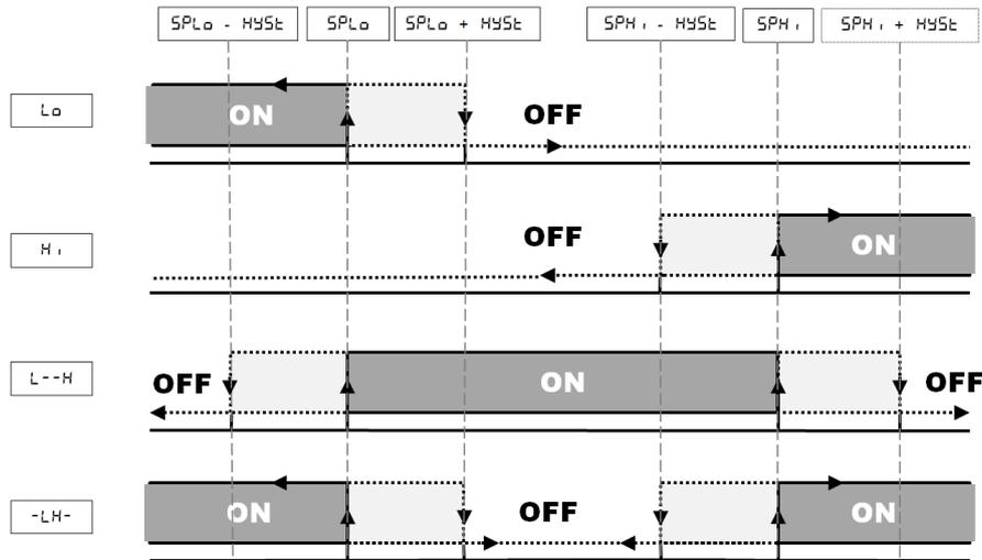
Figure 23 – Alarm output activation and deactivation
