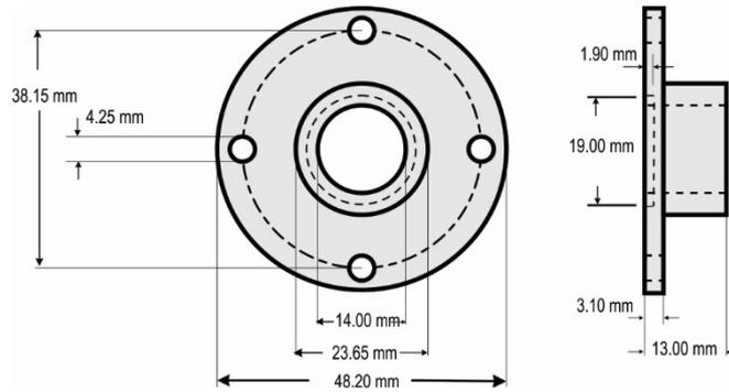
Figure 16 – Flange for mounting DM model
