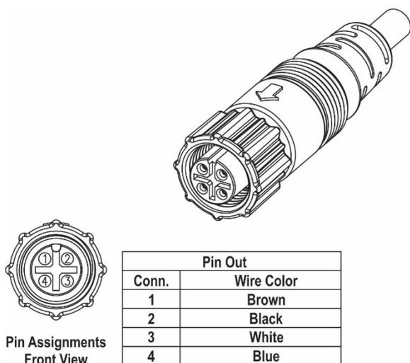
Fig. 7 – Connecting pins for M12 cable mounting
