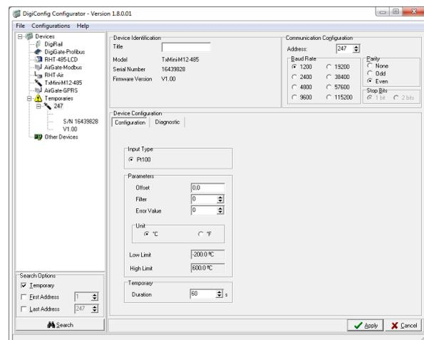
Fig. 1 - TxMini-M12-485 configuration screen in **DigiConfig** software
