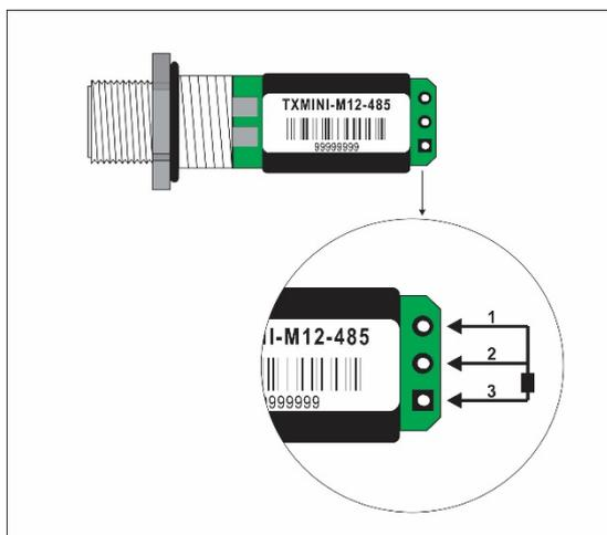
Fig. 6 - Pt100 sensor connection for the model **without** connector
