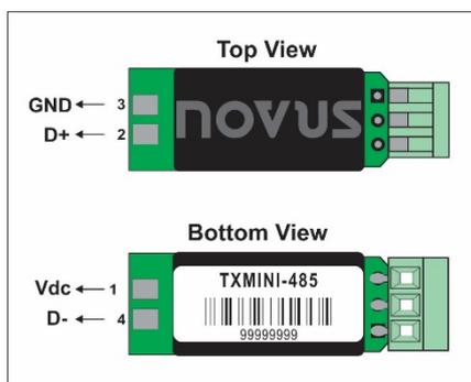
Fig. 4 - Connection diagram for the model without M12
