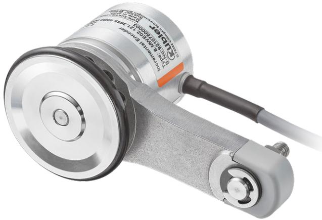
The MWE02 measuring wheel system is the ideal solution for reliable speed, position and distance measurement in applications with linear movements. These are recorded rotationally via the measuring wheel with attached encoder and converted into measurement data.
