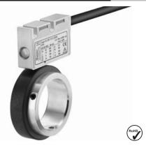
Thanks to its installation depth of only 16 mm, the bearingless magnetic rotary encoder RLI20, comprising a magnetic ring and sensor head, is ideally suited for plants and machinery where space is very tight. The non-contact measuring principle allows for error-free use even under harsh environmental conditions, as well as ensuring a long service life.
