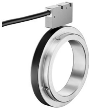
Thanks to its installation depth of min. 10 mm, the bearingless magnetic rotary encoder RLI500, comprising a magnetic ring and sensor head, is ideally suited for plants and machinery where space is very tight. The non-contact measuring principle allows for error-free use even under harsh environmental conditions, as well as ensuring a long service life. In contrast to our measuring system RLI200, a single zero pulse is also implemented here.
