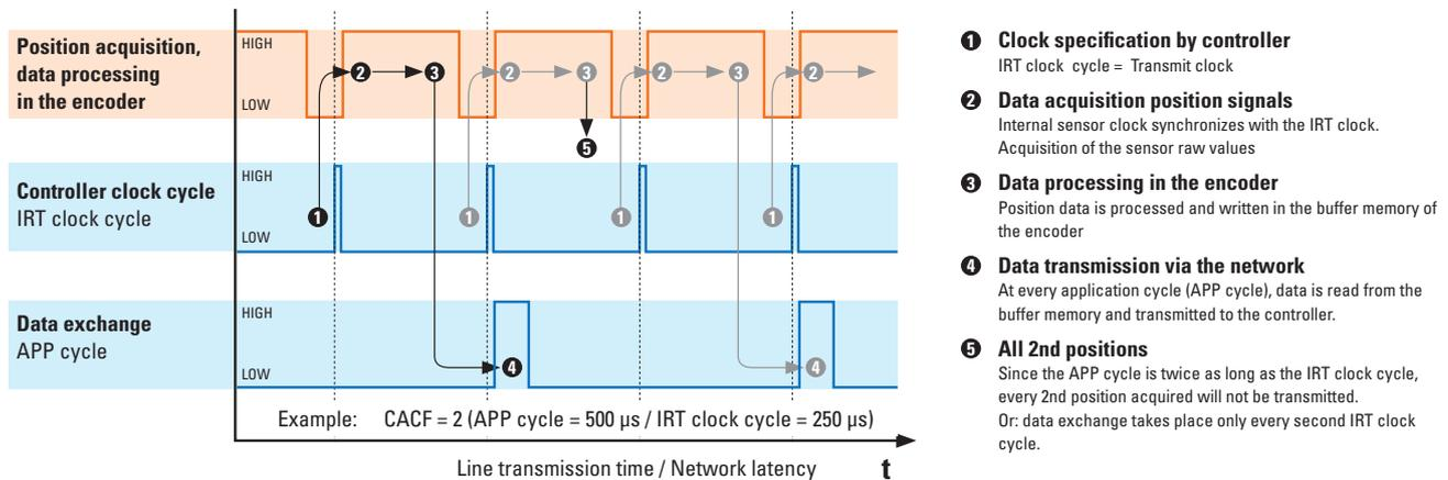
When receiving the IRT clock signal, the sensor starts reading its current measured point. This raw value is processed internally (e.g. scaling, speed calculation, etc.) and stored in a buffer memory.
