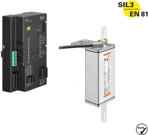
To trigger electromechanical safety gears, the SIL3-certified sensor Ants LES03 can be combined with the SIL3-certified Safety Gear Trigger SGT02. This means that classic mechanical solutions with all the relevant components can be replaced. This reduces both the complexity in the installation process and the number of components in the safety circuit of the elevator system.
