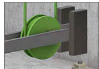
Tensioning device for overspeed governor
