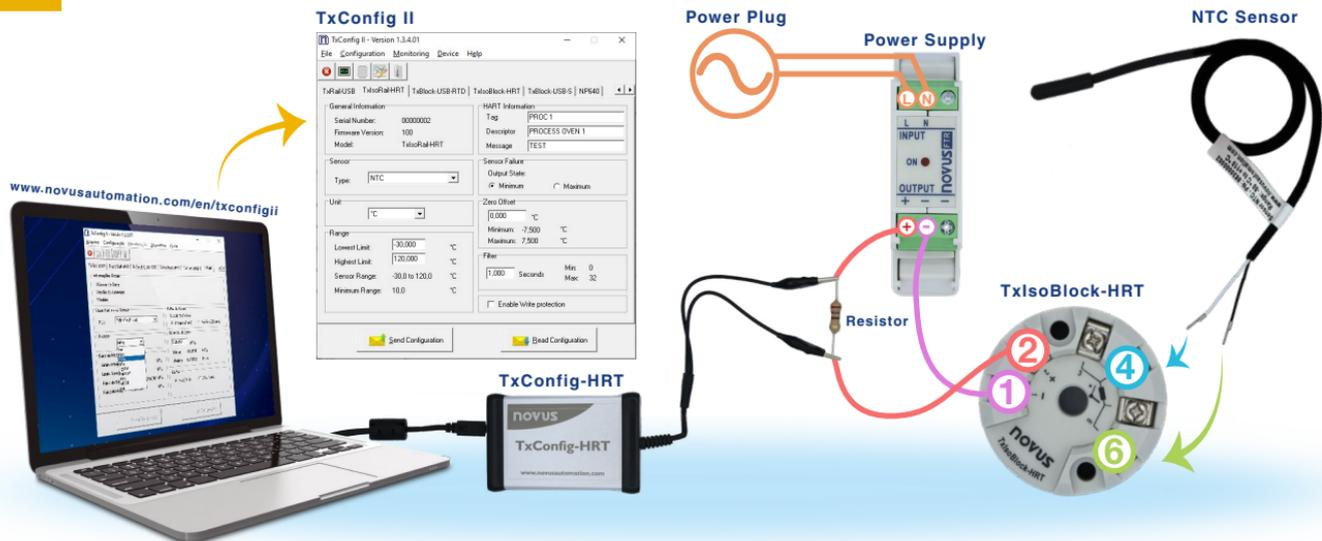
Install TxConfig II software in your computer and connect TxConfig-HRT interface to install the drivers.
