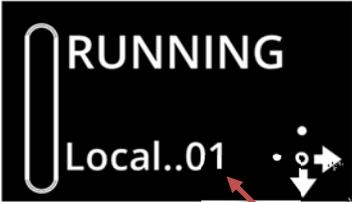
Modbus address of connected unit
