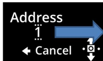
Use UP / DOWN keys to select address. Press centre to confirm
