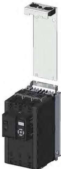
Step 2. Loosen the two lower mounting screws (2a) and slide the fan assembly downward between the mounting bracket and the heatsink fins (2b)
